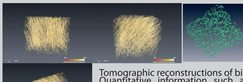
Tomographic reconstructions of biomaterials. Quantitative information such as porosity, specific surface area and pore size distribution have been obtained
