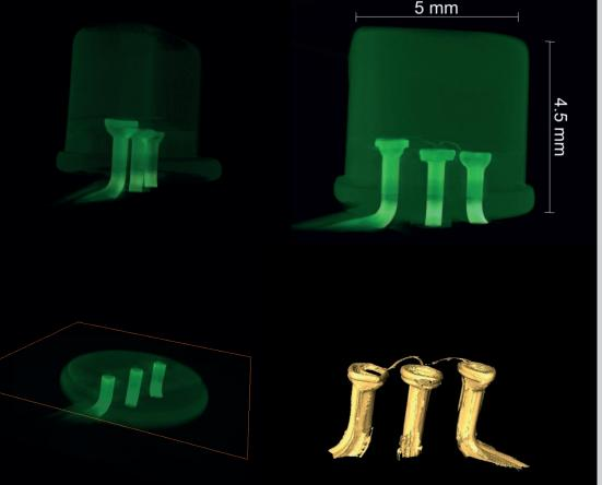
Comparison of resolution and artefacts appearance: Microtomogarphic crossection of a resolution phantom a) Microtomographic system based on a laboratory source (IFJ PAN)
